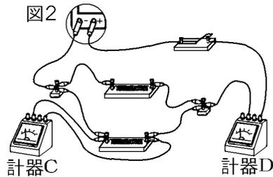
[電流計・電圧計のつなぎ方と回路図]
